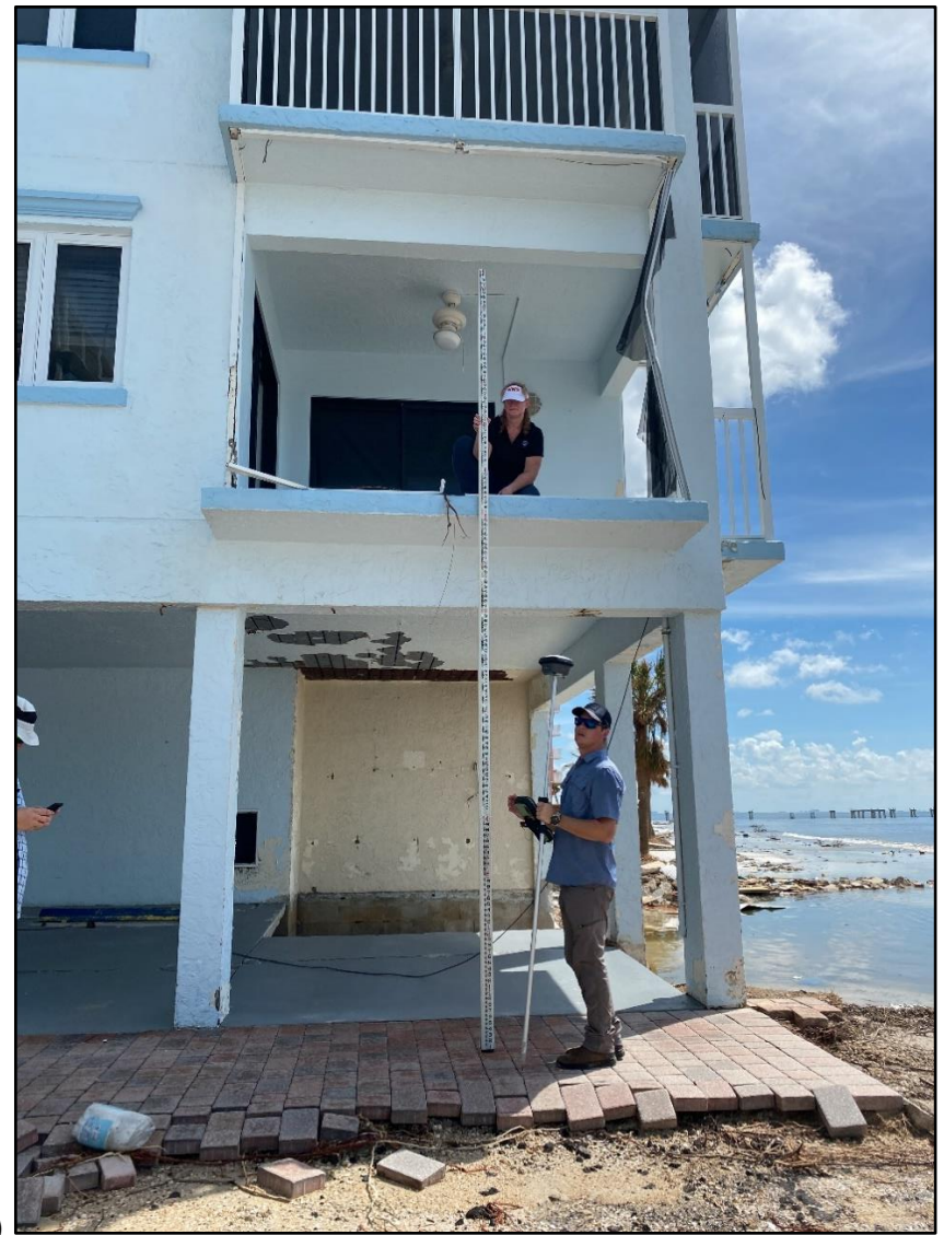
Figure 12. (a) Storm surge high water mark in bathroom cabinet on the second-story of a beachfront structure in Fort Myers Beach. (b) NWS survey team extrapolating the high water mark to the outside of the home to survey its elevation of approximately 12 ft above the brick foundation and 15 ft above MHHW. Images courtesy of the NWS.
